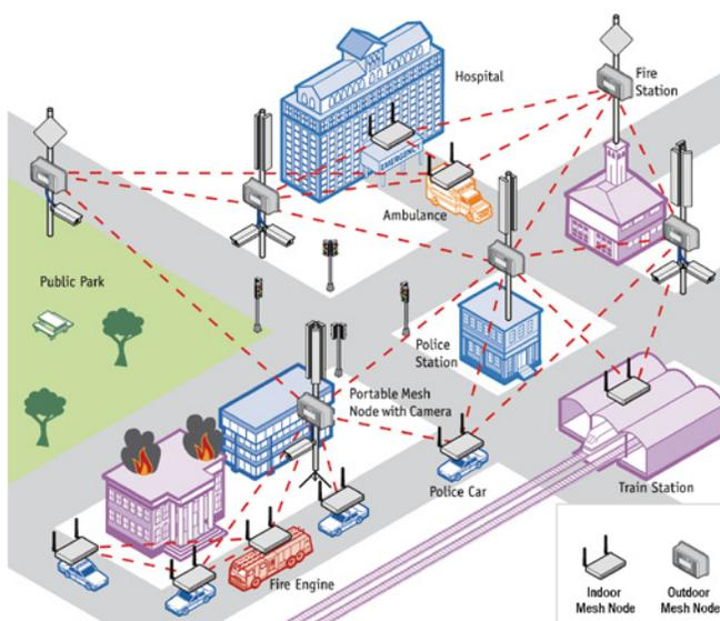
The Firetide HotPort® wireless mesh network allows indoor, outdoor, and mobile video surveillance without costly backbone cabling between walls and buildings. The mesh network forms itself and is self-healing. If one link is blocked or if a node is removed, the mesh will reroute traffic over a different path.
