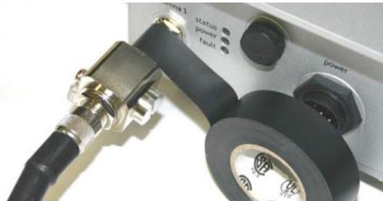
4. Repeat for the antenna cable to arrestor connection.
