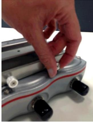
2. Remove the hook attachment plate.
