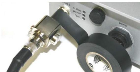
5. Repeat for the antenna cable to arrestor connection.
