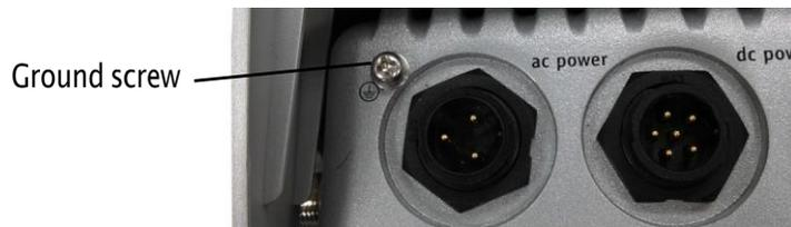
4. Insert the ground lug for the enclosure.
