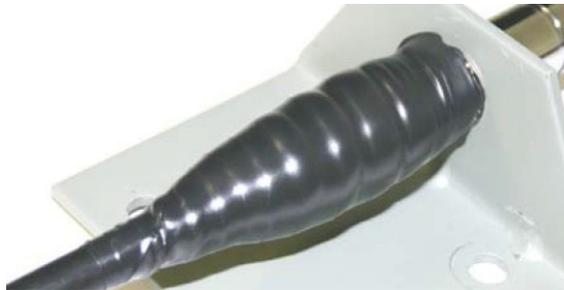
8. Wrap a second layer of electrical tape over the first layer of electrical tape. The antenna connector is ready for installation in an outdoor environment.
