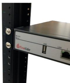
4. Use two screws for each bracket to attach them to the rack rails.
