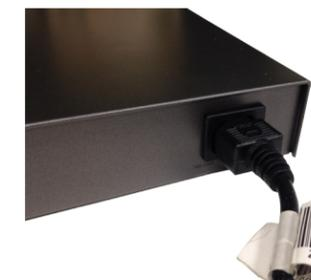
When you supply power to the FMC 2000 appliance, the power LED (green) and test LED (yellow) come on. After two minutes, the test LED turns off, and the appliance is ready for use.
