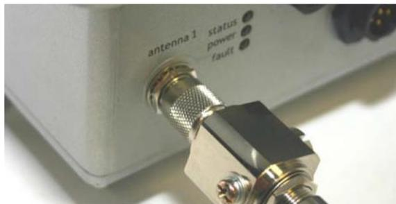
4. Wrap a layer of electrical tape (sticky side out) over the arrestor to node connector and wrap approximately 2.5 cm (1 inch) of cable. Overlap the tape by 40% with each turn.
