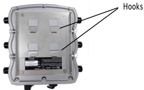
The installation is correct if the node does not easily move from side to side, and the connectors are oriented to the ground.
